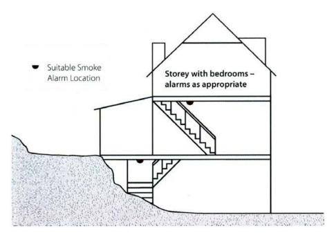
Smoke alarms should be installed on or near the ceiling, with special care taken to avoid installation in the following areas –
