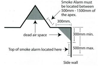
If it is not practicable for a smoke alarm to be installed at the location required under this regulation, the smoke alarm may be installed at another location that will provide a warning to occupants of the residential premises or moveable dwelling, for example a smoke alarm that is regularly activated by steam from a bathroom or smoke or fumes from a kitchen may be moved to another appropriate location.
